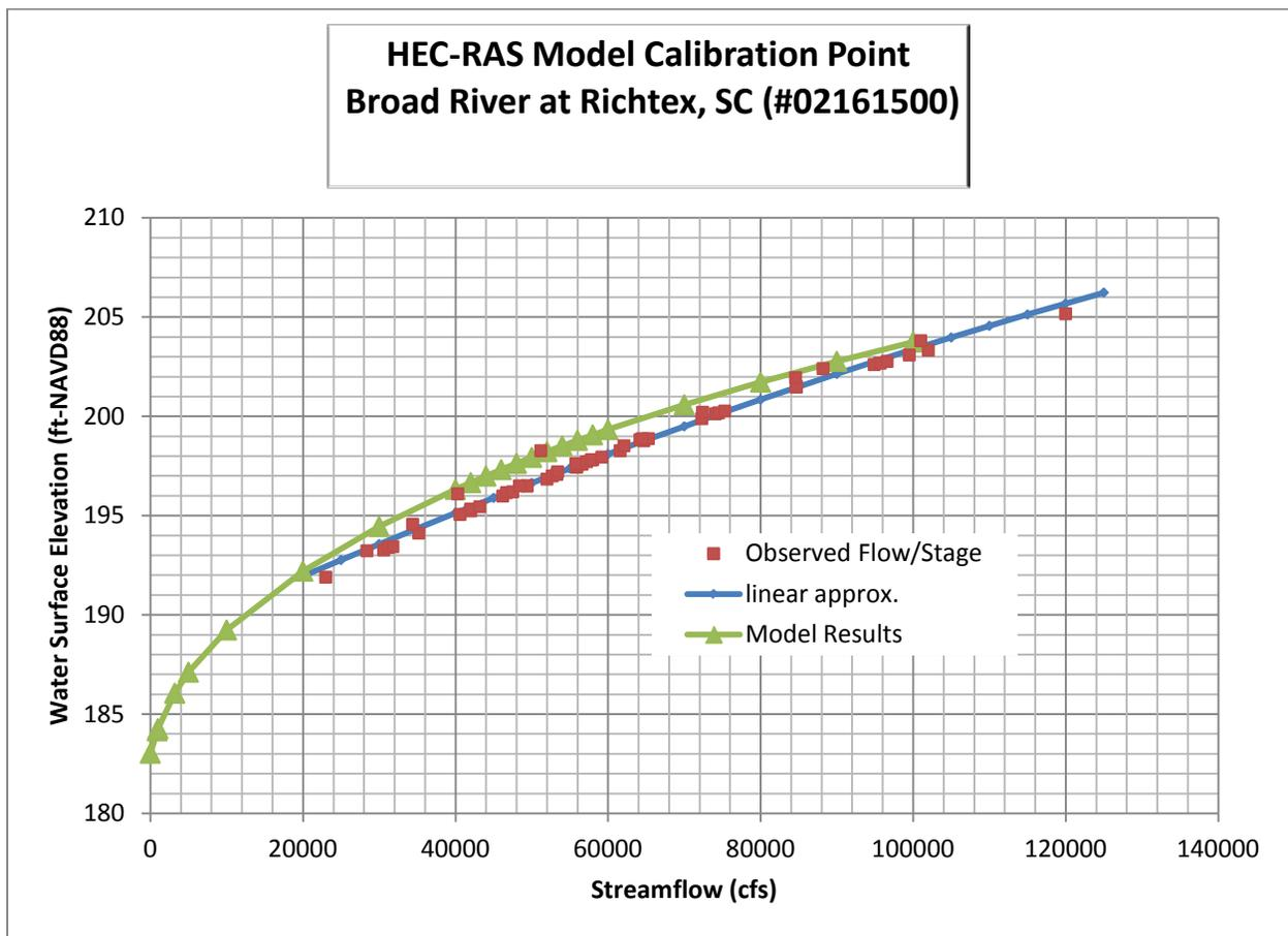
**FIGURE 3-6 HEC-RAS CALIBRATION AT RICHTEX GAGE SITE**
